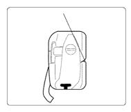
PULL THREAD THROUGH SLIT OF CASE AS SHOWN.
