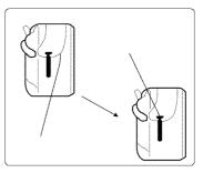
PULL THREAD UNDER TENSION SPRING AND THROUGH THE OPENING AS SHOWN ABOVE.
